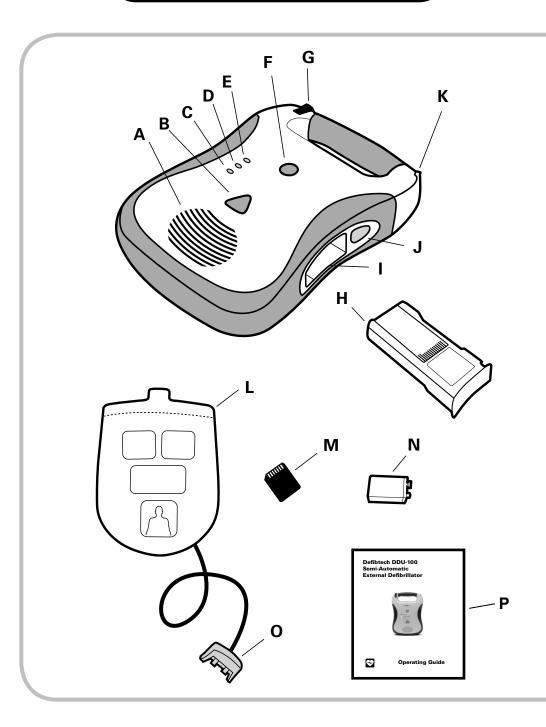
**A.** *Speaker.* The speaker projects the voice prompts when the AED is on. The speaker also emits a "beep" when the unit is in standby mode and has detected a condition that requires operator attention.
