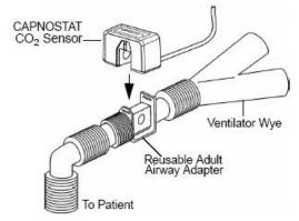
Figure 6.32 Attach Airway Adapter to Airway Circuit
