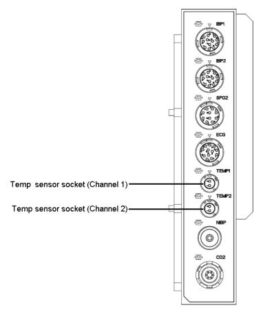
Figure 6.22 Temp Sensor Socket
