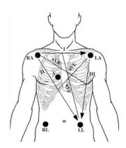
Figure 6.3 Placement of 5-Lead Electrodes
