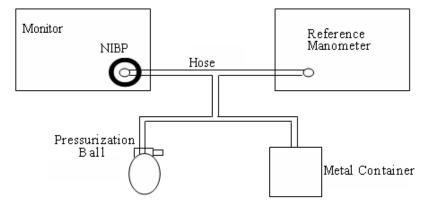
Figure 6.21 NIBP Calibration Diagram
