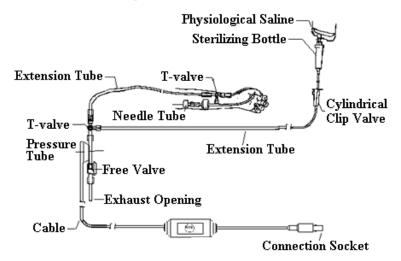
Figure 6.24 IBP Monitor Connection Diagram
