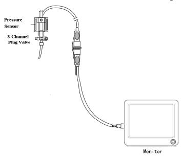
Figure 6.28 IBP Zero Calibration
