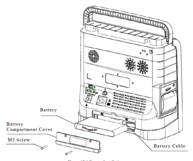
Figure 12.1 Battery Installation
