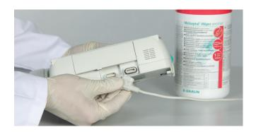
All electronic connections have to be disconnected from the power grid before cleaning or disinfection.
