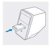
(4) Insert cartridge. The test starts automatically.
