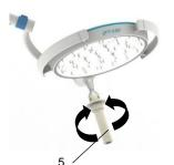
Focus the light field by turning the handle (5)
