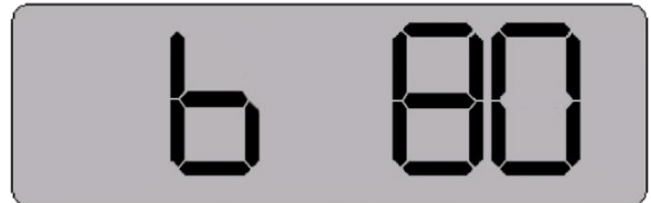
Fig. 3-6 Battery capacity of 80 %
