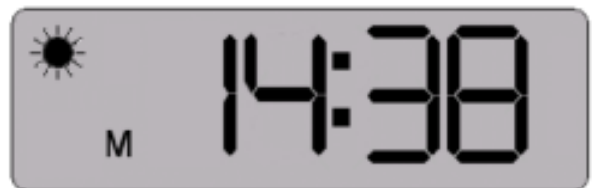
Fig. 3-7 Example: Display after successful self-test ( M = BP data in memory, ☀ measuring phase: day)
