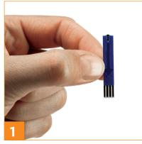
Remove test strip and place into analyser.
