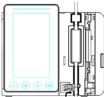
(4) Close the pump door, then pop up the infusion tube selection interface, indicating that the infusion tube is installed correctly. Otherwise you need to reinstall
