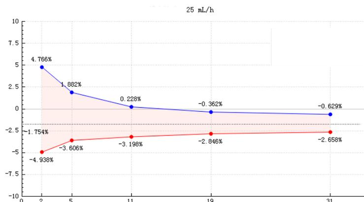
**Graph 4 Trumpet curve: Percentage variation  $E_p$  against observation window duration  $P$  (min) and the overall mean percentage error  $A$  plotted from data gathered during the second hour of the test period**
