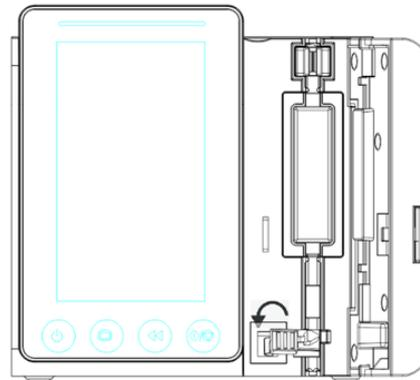
(3) Gently pull the infusion tube, straighten it, and fix the infusion tubing the tube groove at both ends from top to bottom, and close the anti-free flow clip to clamp the infusion tube.
