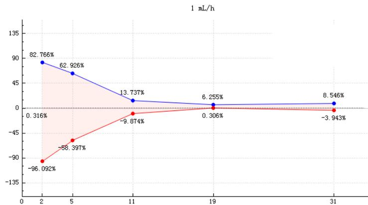
**Graph 3 Trumpet curve: Percentage variation  $E_p$  against observation window duration  $P$  (min) and the overall mean percentage error  $A$  plotted from data gathered during the second hour of the test period**
