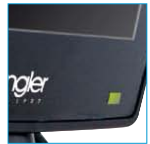
Low battery indicator
